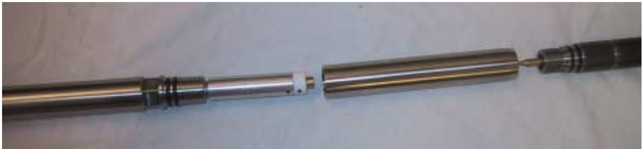
Downhole Tool, SRO Transmitter, GO to Recorder Adapter and GO Cable Head
